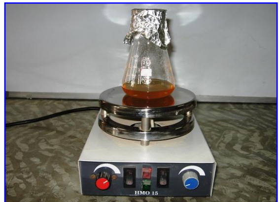
2- Dehydrated medium is dissolved in a measured amount of distilled water and pH
