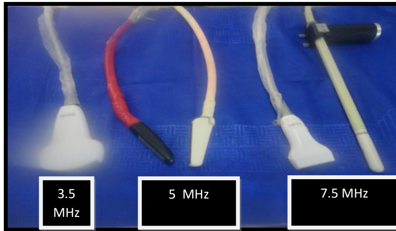
Figure show different probes equipped with the scanner system(3.5, 5, 7.5 MHz).
